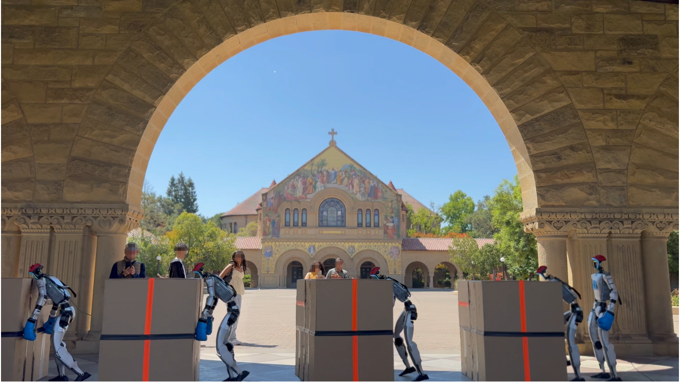
Fig. 1: We present VisualMimic, a visual sim-to-real framework for whole-body humanoid loco-manipulation. Videos are available at visualmimic.github.io .
